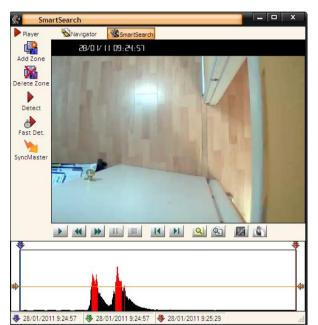
After selecting the area where the motion is to be assessed, the "Detect" button must be clicked on (it analyzes all the images of the recording) or "Fast Detection" (it analyzes one of every two recorded images)
