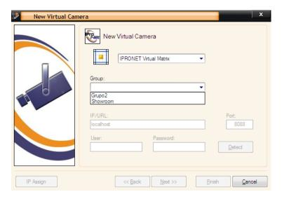
The virtual cameras are different combinations of cameras and information where a video "re-encoder" system allows you to merge into a single video stream images from multiple cameras, including from information sources other than the video.
