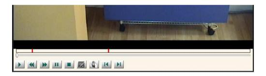
The other buttons show the usual controls of a playback system: play, rewind, fast forward, pause and stop recording. It can be fast-forward or rewind, minute by minute (Page Up, Page Down), second by second (cursor back and forth) and even frame by frame (by clicking on the image).
